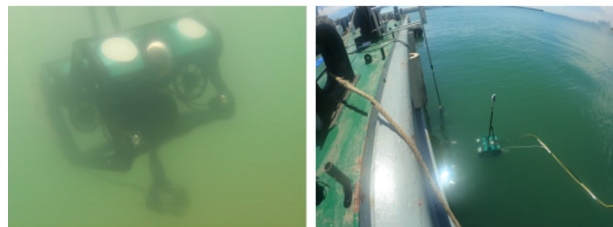
(e) AUV 水下工作 (f) 导引回收实拍图 (e) Underwater operation of the AUV (f) On-site photo of docking
